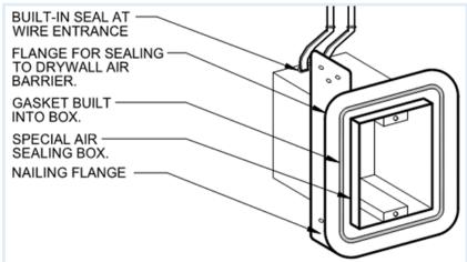
This detail is showing an air-sealed box.
