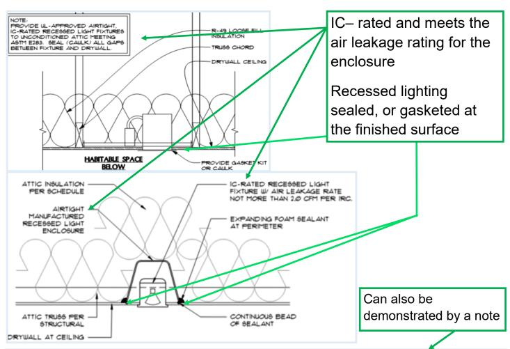
RECESSED LIGHTING INSTALLED IN THE THERMAL ENVELOPE SHALL BE SEALED WITH A GASKET OR CAULK BETWEEN THE HOUSING AND THE INTERIOR WALL OR CEILING COVERING. BE IC-RATED AND LABELED AS HAVING AN AIR LEAKAGE RATE NOT MORE THAN 2.0 CFM PER IRC.
