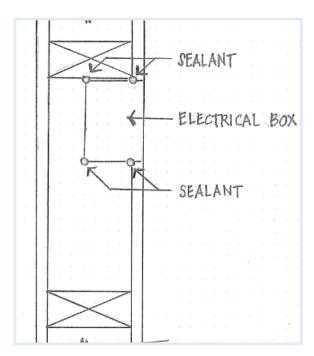
This detail is showing self sealing of electrical box.
