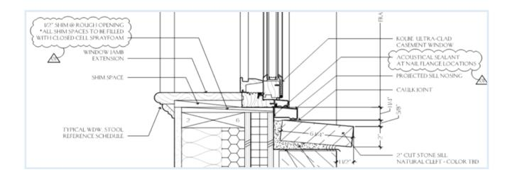
Openings between window and door assemblies and their respective jambs and framing shall be sealed and insulated with sprayed foam with a thermal resistance of R-3 per-inch minimum.
