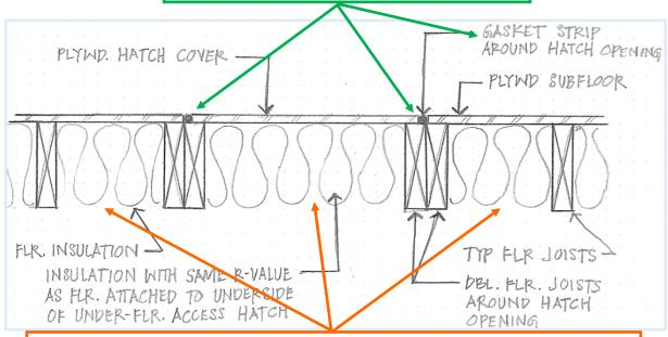
Air barrier is missing to separate the unconditioned space from the conditioned with it in alignment of the insulation.
