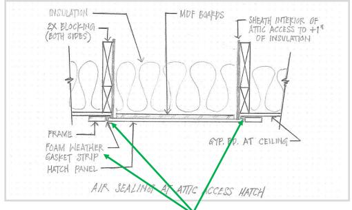
Sealing shown at edges of opening with a gasket
