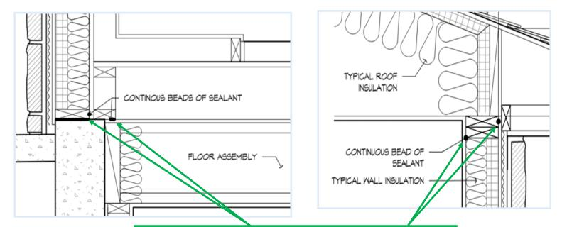
Sealing provided at bottom (sill) plate and at top plate
