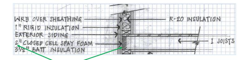
Closed cell spray foam can be considered an air barrier if installed to a certain thickness.
