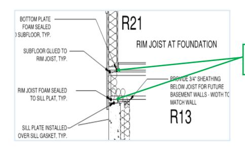
Calls out for the sill plate and subfloor to be sealed
