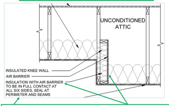
Air sealing is called out and an air barrier is provided and called out
