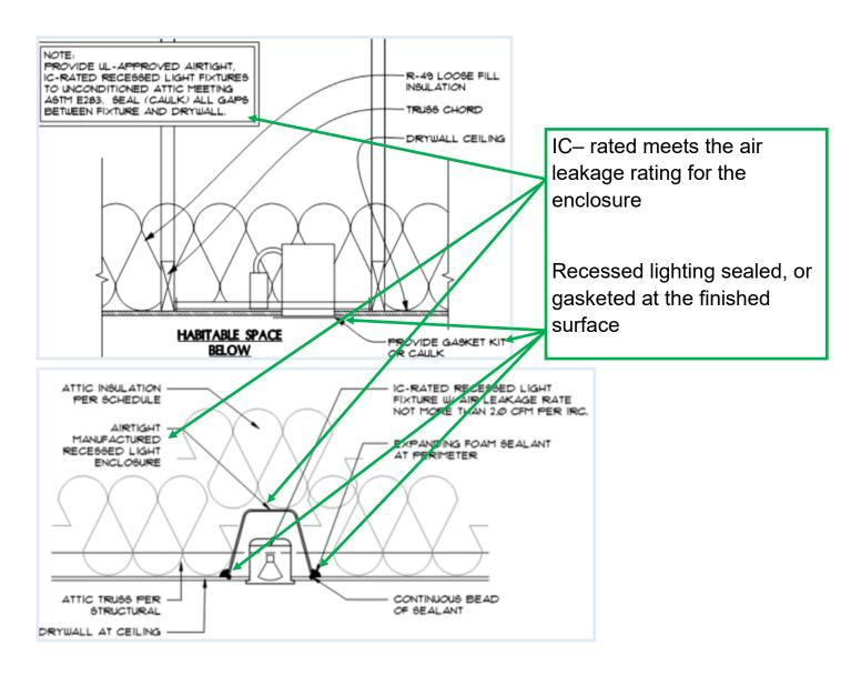
RECESSED LIGHTING INSTALLED IN THE THERMAL ENVELOPE SHALL BE SEALED WITH A GASKET OR CAULK BETWEEN THE HOUSING AND THE INTERIOR WALL OR CEILING COVERING, BE IC-RATED AND LABELED AS HAVING AN AIR LEAKAGE RATE NOT MORE THAN 2.0 CFM PER IRC
